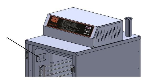
2. Check the product door hinges and the product door latches. Tighten screws and align as needed.
